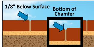
If desired, "strike the joint" using a mason jointing tool to smooth the joints after all previous steps have been completed.
