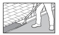
**Step 1:** Prior to compacting the pavers or natural stone, remove bedding layer (sand or chips) that extends outside the perimeter of the project. For optimal, performance, remove all of the bedding material down to the base material.
