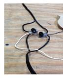
Note: When you reach the last light on the string, you will only use two holes on each connector as shown.
