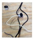
8. Examine the connectors and note there are three holes in each. The outside holes are for the power cable and the middle hole is for the lead from the fixture. Cut one side of the split power supply cable. There is no need to strip the insulation. Place each end of the cut power cable into the two outside holes in the connector. Push one of the cables
